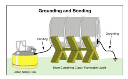
Bonding connects two or more pieces of conductive equipment together using wires, cables, or other connecters in order to equalize their static charge. Sparks cannot occur between objects that are at the same electrostatic potential. Containers need to be connected even if they are touching, because paint or other coatings may reduce the conductivity. Simply touching another object does not guarantee an effective connection for static charge to transfer.
